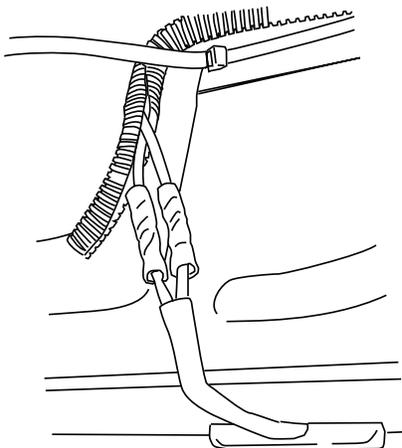
Close and wrap conduit with electrical tape. Secure all loose wires with cable ties. Pull lamp wires upward to avoid any wire snagging.
