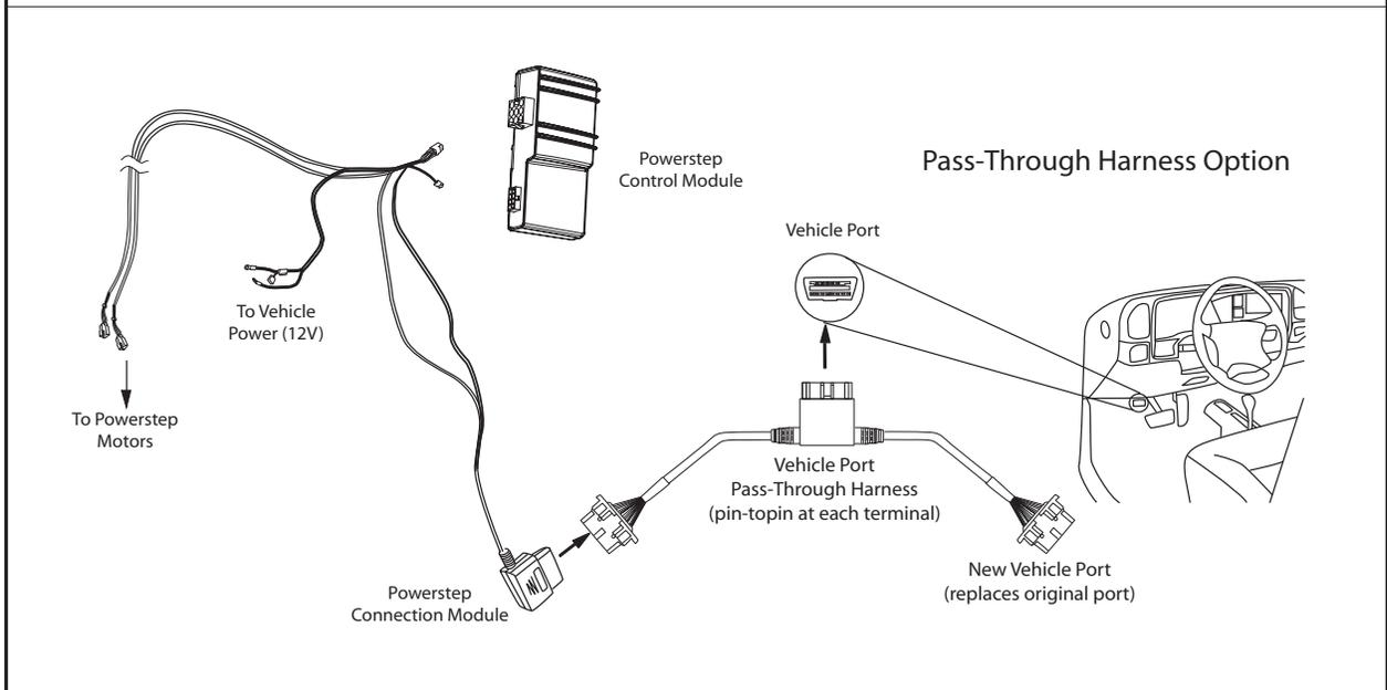
Check that all doors activate the Power Step and the LED Lights work when doors open and close. Reinstall any remaining trim panels.
